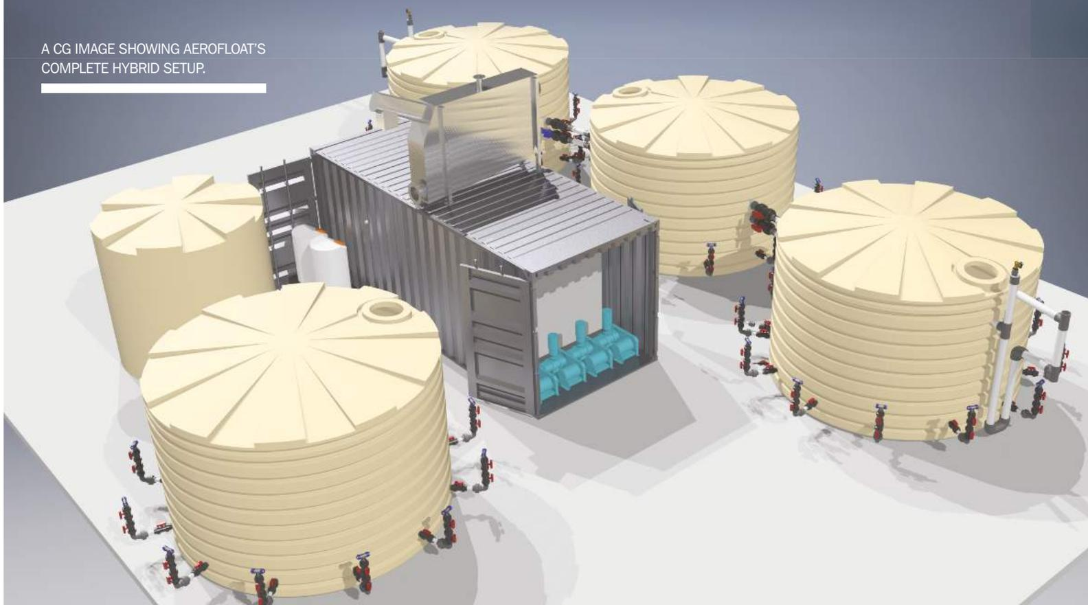
with excess biomass, flows to one or more tanks called Sequence Batch Reactors (SBRs), which again use multiple blowers and Aerofloat's lances to provide optimal and intermittent aeration and mixing.
