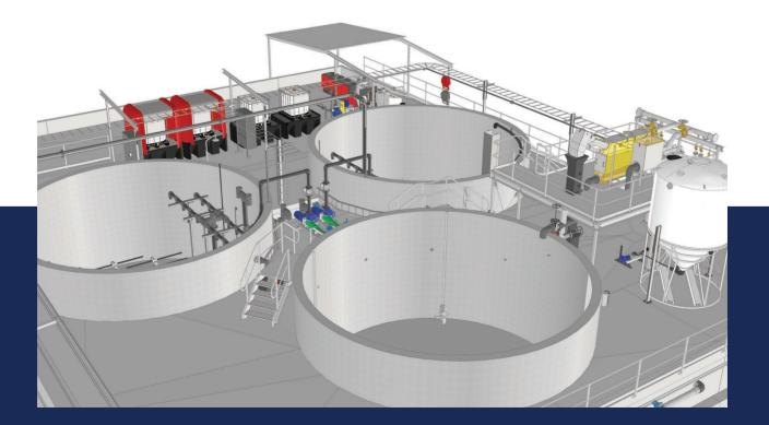
In most conventional activated sludge plants, mixed liquor is continuously pumped back to the anoxic reactor and then recycles back to the activated sludge reactor. In Aerofloat's Hybrid SBR process, the mixed liquor is pumped forward from the Anoxic/FBR to the SBRs at flow rates of approximately 4 times the average daily flow (ADVVF) during the aeration and mix phase in the SBRs, and mixed liquor recycles back to the Anoxic/FBR.
